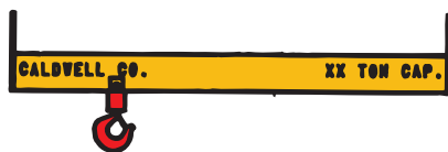
OPTION A Off-set hook for hoists of different capacities.
