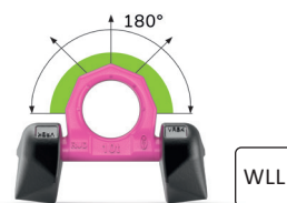
WLL angle in load ring plane
