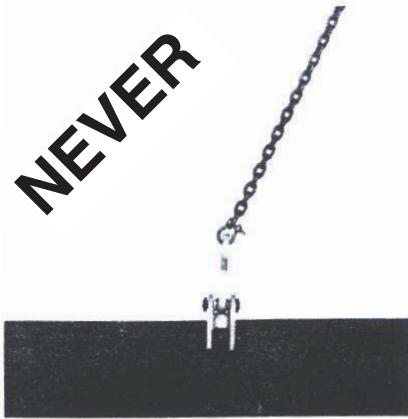
Photograph G (typical) Excessive side loading.
