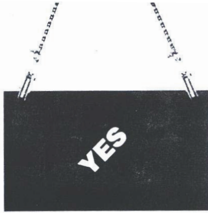
Photograph H Clamps in line with sling
