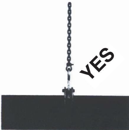
Photograph E (typical) Sling directly above and in line with the lifting shackle.
