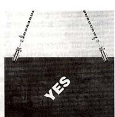
Photograph H. (Typical) Clamps in line with sling. (J and JA only)
