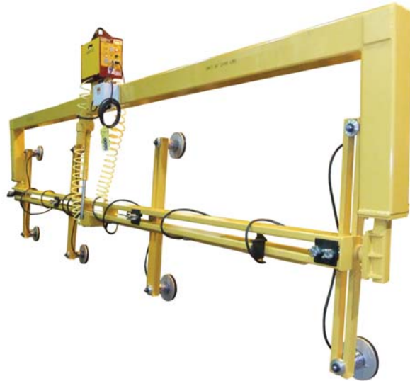
Electric upender shown at 90° position.
